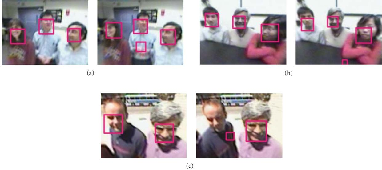
FIGURE 10: Samples of indoor and outdoor test video clips for counting the face detection rates and false positives.
