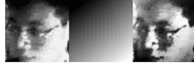
FIGURE 4: Illumination compensation of the face video. The left is the originally extracted face image, the middle is the intensity plane fitted to the intensity grade of the original face image, and the right is the compensated and equalized face image.
