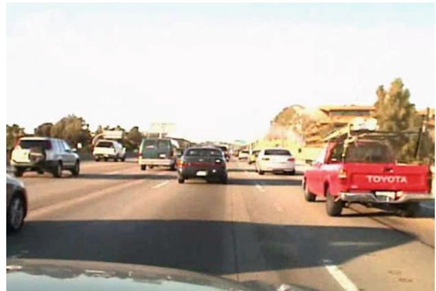
**Fig. 4** Example from *LISA\_2009\_Dense* validation set. The dataset consists of 1,600 consecutive frames, captured during rush hour, over a distance of roughly 2 km. The ground-truth dataset is publicly available to the academic and research communities at <http://cvrr.ucsd.edu/LISA/index.html>
